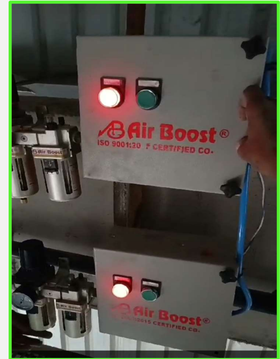
After Raw material hopper – Installation of Polymer liner and Air blaster to avoid jamming and to have a continuous flow of material
