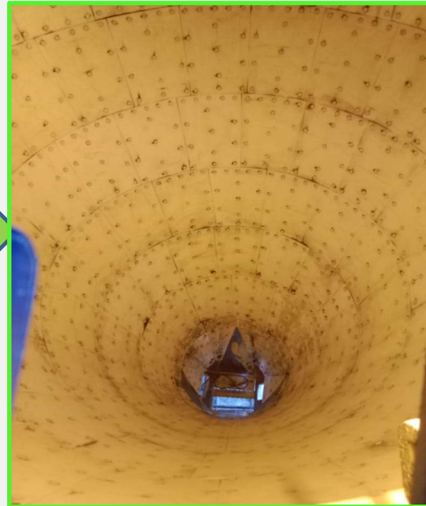
After Raw material hopper – Installation of Polymer liner and Air blaster to avoid jamming and to have a continuous flow of material
